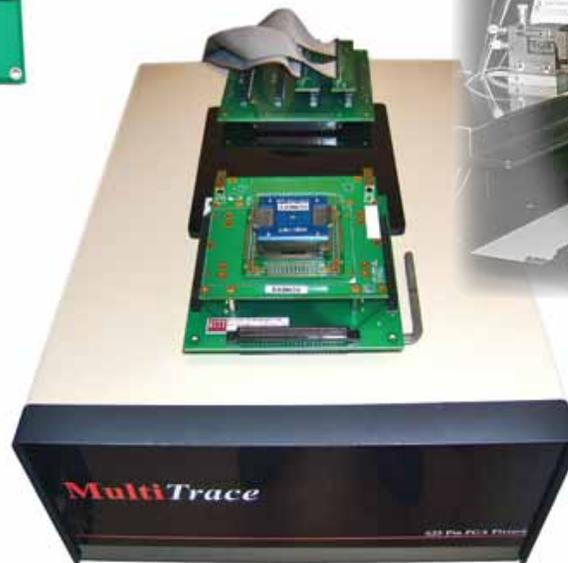
950 Dedicated Fixture Mounted on a RTI MultiTrace Test System and Connected to a Black Box For Microscope Use
