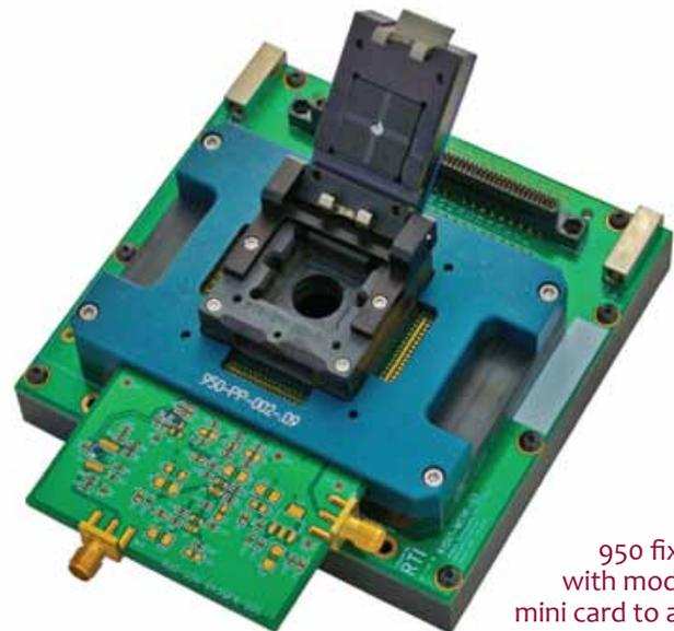
950 fixture with modified mini card to allow RF measurements on a hybrid RF module.
