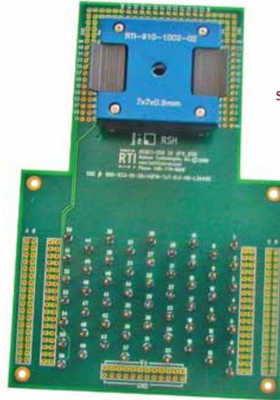
Mini card with extension to allow access to all DUT pins. Can be used stand-alone or with the 950 base.
