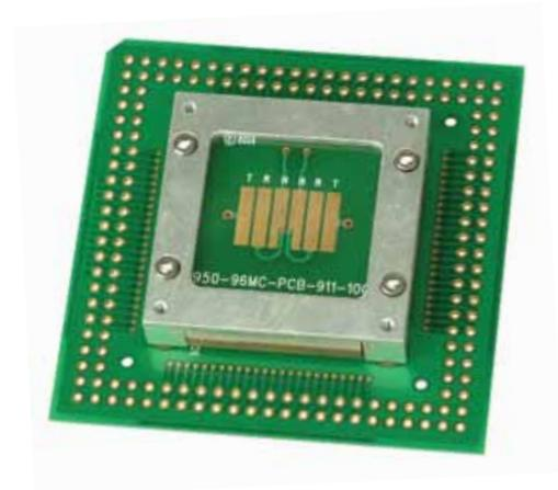
Bottom of 950 mini card shown here with contacts for heated socket base
